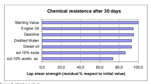
Support: stainless steel Curing cycle: 2hrs at 80°C
