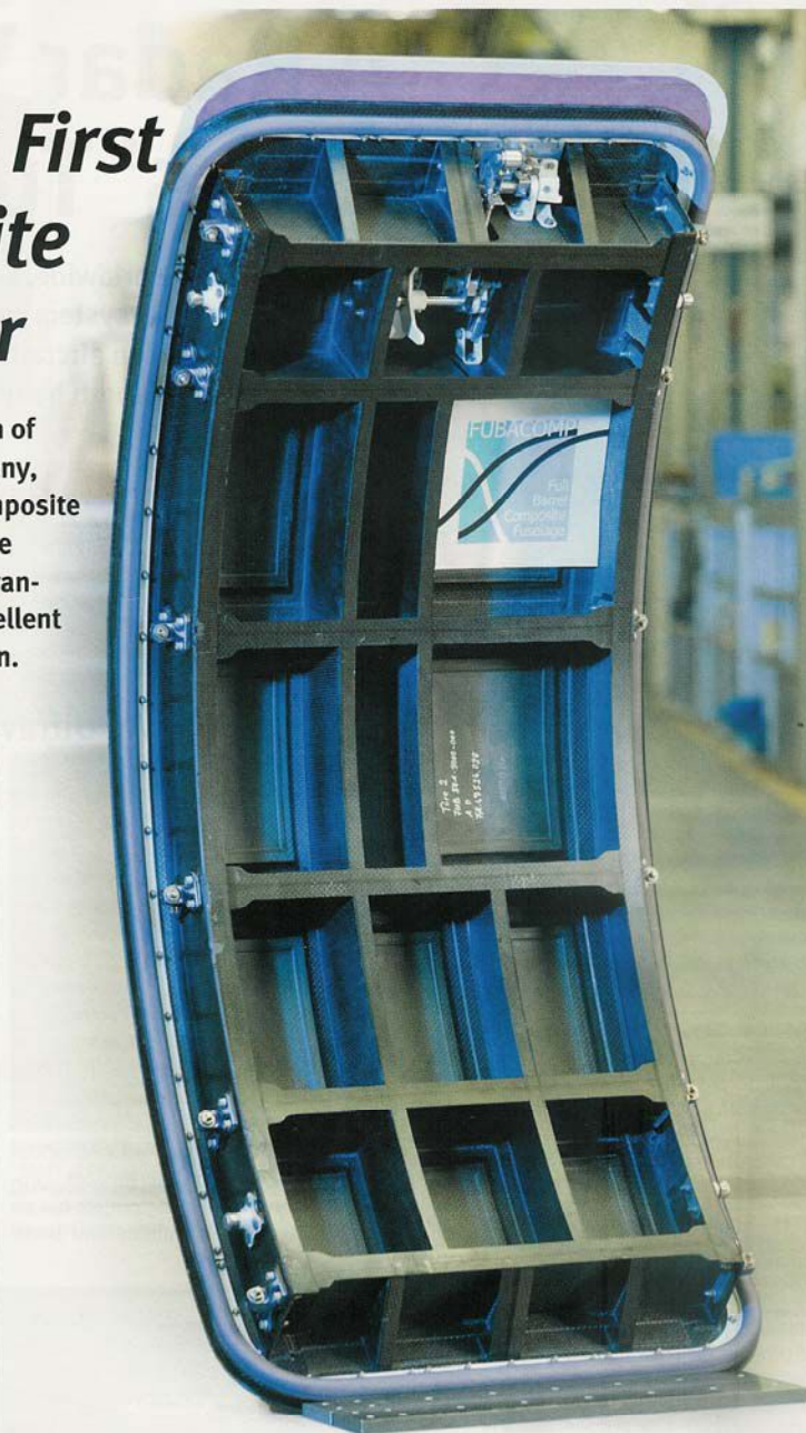
The all-composites aircraft door made by Eurocopter is called 'monolithic' because all its components (spars, frames, skin) are produced and joined in a single molding operation.
