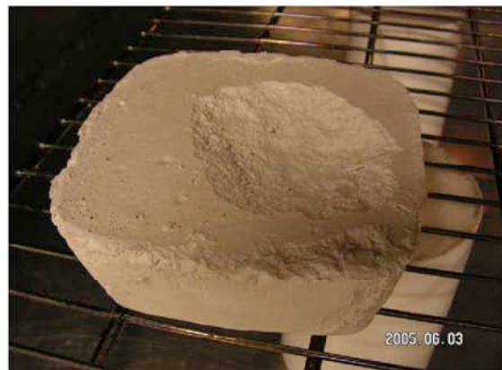
Figure 7: destroyed specimen at 300W/m 3
