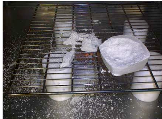
Figure 6: destroyed specimen at 400 W/m 3
